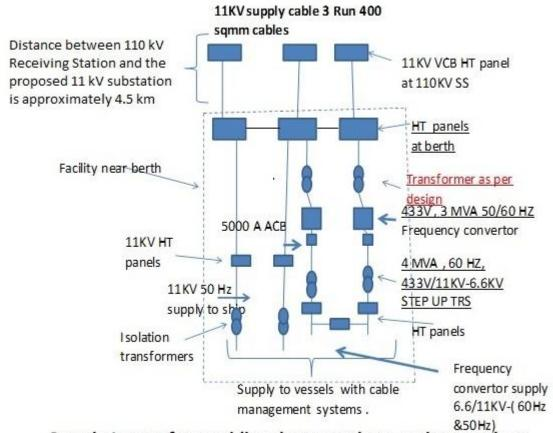
Sample Layout for providing shore supply to cruise vessels at Harbour
