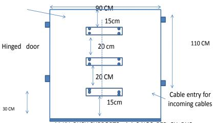
11 KV BUSH SUPPORTS mini. 2 NOS .PER CU. BUS BAR, CABLES 2NOS. 3C 240 SQMM AND 1 NO. 35X3+16x3 COPPER CABLE. (Dimension given is only approximate and shall be done as per STD)
