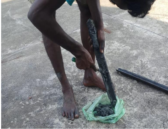
Figure 26 A view of sample collection from SPT spoon sampler
