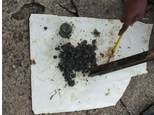
Figure 26 A view of sample collection from SPT spoon sampler
