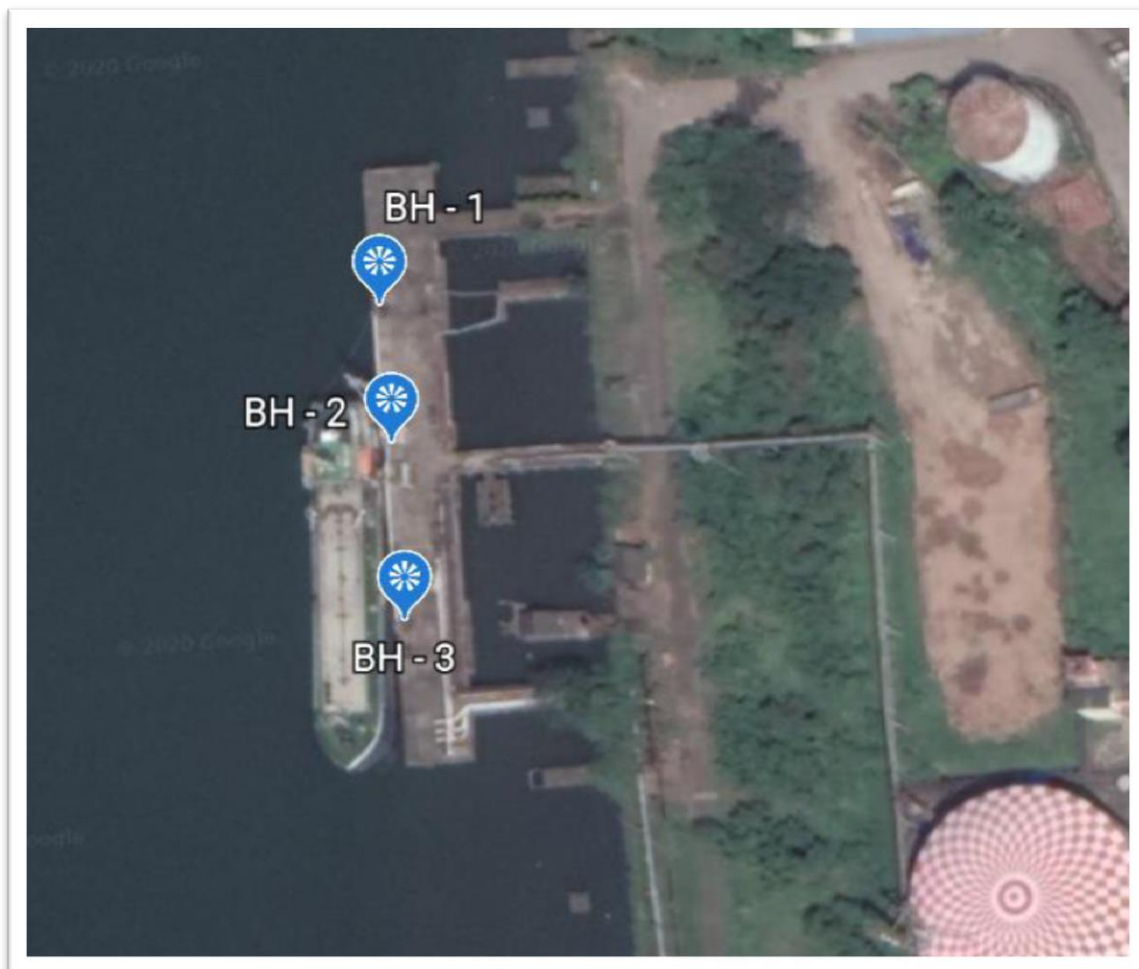
Figure 4.1 Locations of Boreholes at South Coal Berth
